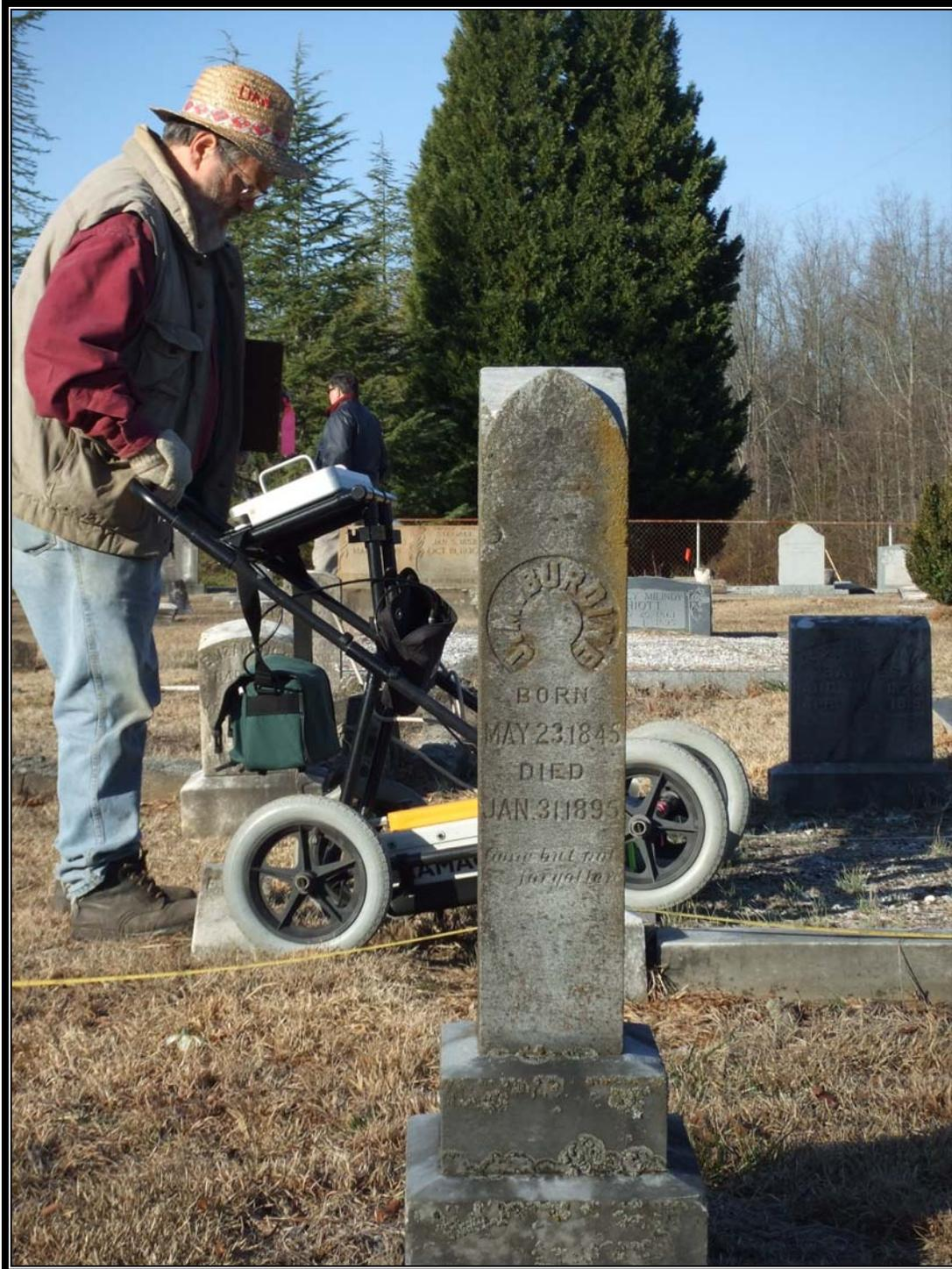
Figure 2. GPR Survey in Progress.
